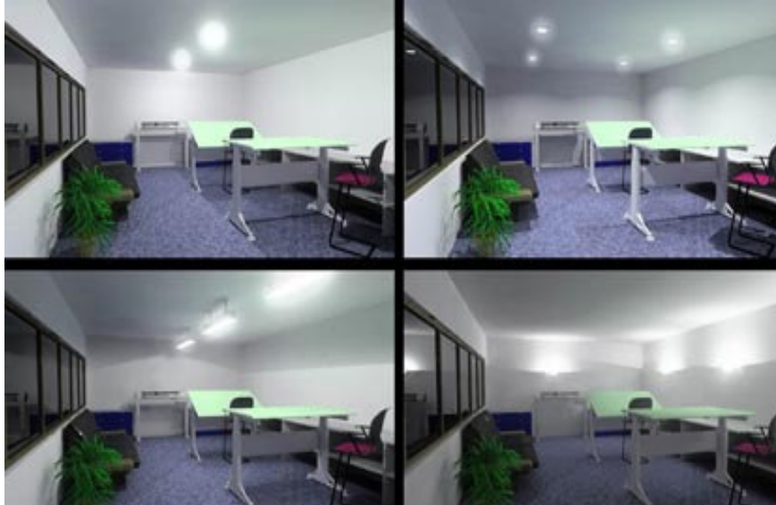
Fig.(5-2) A Simple ECOTECT Model Using RADIANCE to Compare the Effect of Different Lighting Layouts March, Andrews and Raines, Caroline, http://www.squ1.com/ecotect/overview.html accessed 8 / 2003
