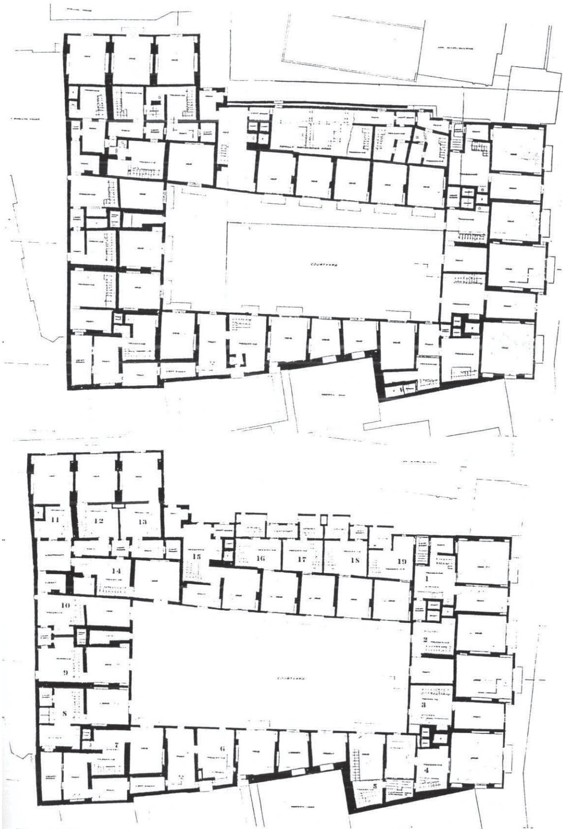
Fig. (48)*: Wakalat Bazaraa, plan of the third floor, present condition and proposal for restoration.
