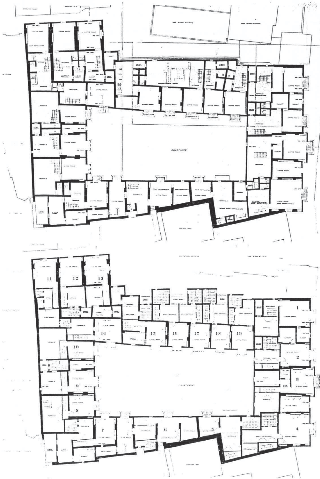
Fig. (49)*: Wakalat Bazaraa, plan of the fourth floor, present condition and proposal for restoration.
