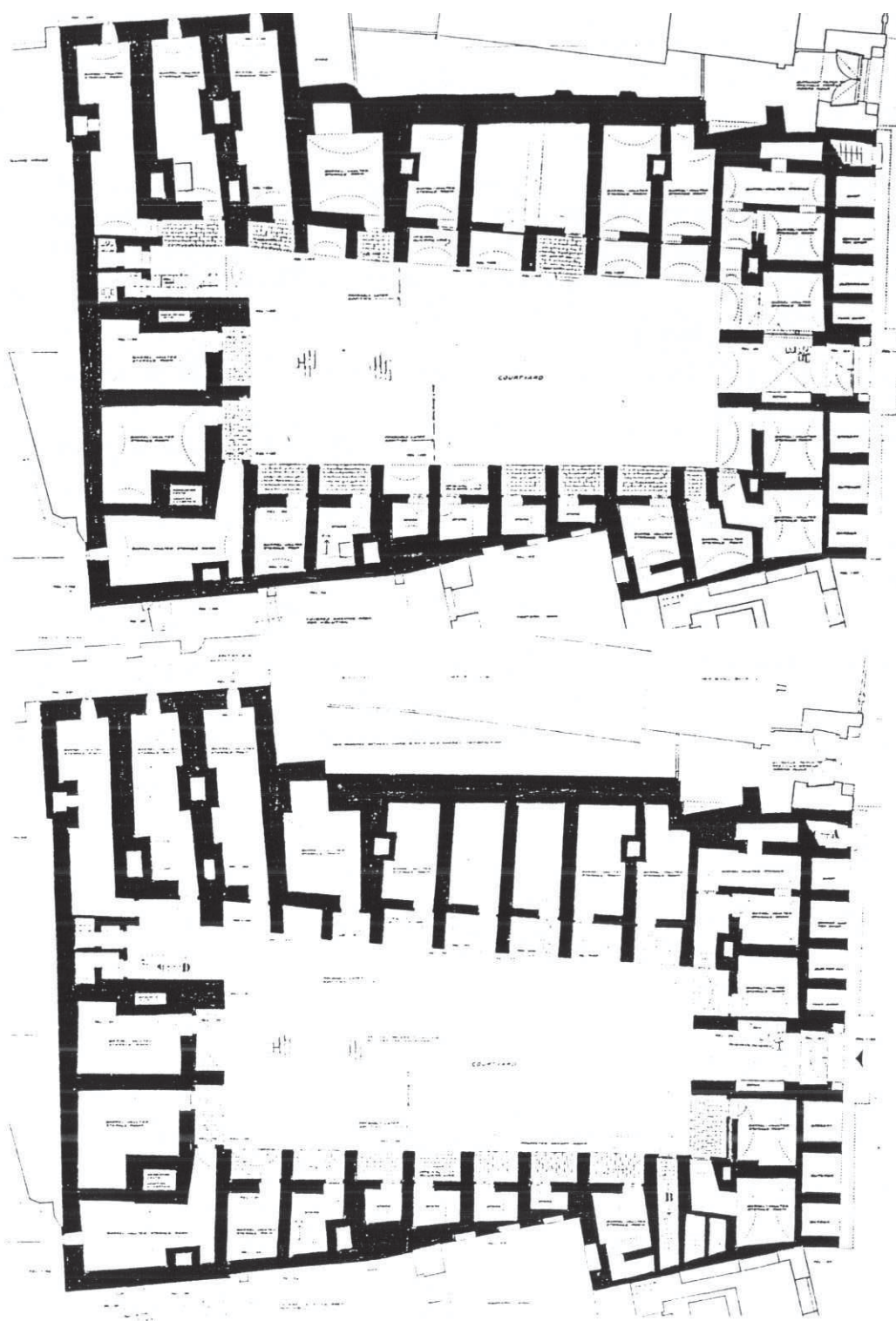
Fig. (45)*: Wakalat Bazaraa, plan of the ground floor, present condition and proposal for restoration.
