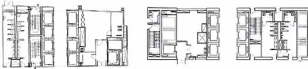
Figure (30) Different examples for cores inside tall buildings
