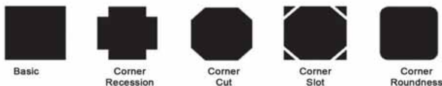
Figure (93) Corner modifications.
