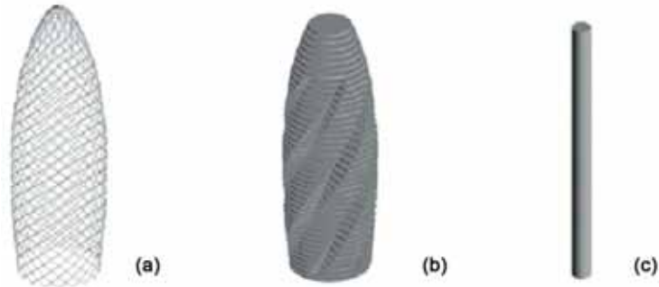
Figure (141) Structural idea. (a) Steel dia-grid, (b) Floor plates, (c) Core Ref: (Bridwell). P.114.
