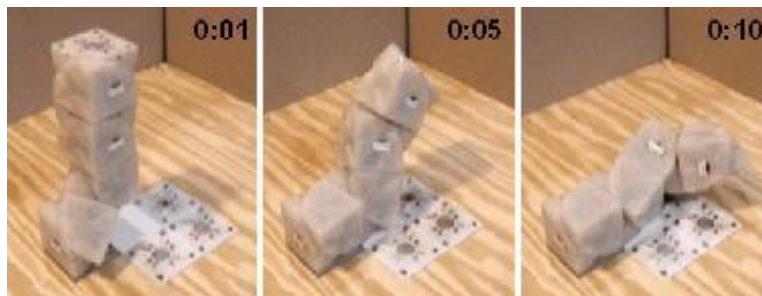
(Fig. 3.5): Hod Lipson and other scientists at the Cornell Computational Synthesis Lab have begun developing multiple types of modular reconfigurable robots and evolutionary robots. These self-replicating prototypes were designed to allow for each object to be able to attach, detach, and reattach to different self-similar faces based on predetermined computational logic. These modular objects are able to connect to each other through electromagnetic connections, and the entire system has the ability to change its physical shape based on how it is programmed.
