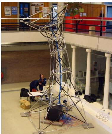
(Fig. 3.30) : The Muscle Tower 2 the structure is flexible enough to move and rotate according to different stimuli .
