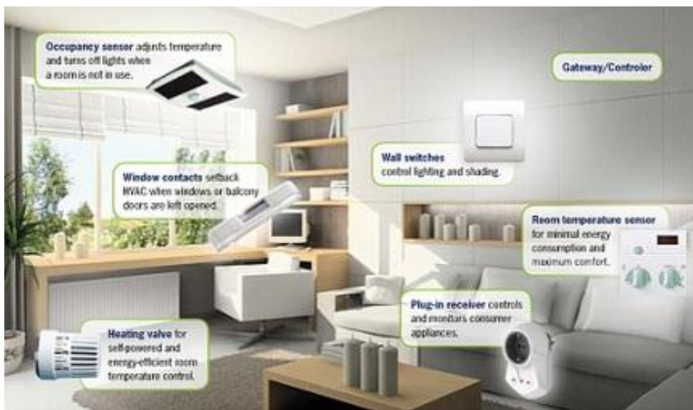
(Fig. 1.37): a home automated environment showing different levels of sensors to capture the different information about its surrounding environment
