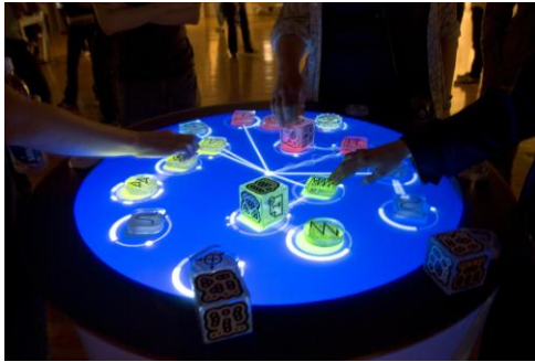
(Fig. 2.12) The “reactable” is a multi-touch surface sound synthesizer. It changes sounds according to the user’s direct manipulations of cubes on the table. It also draws dynamic animations on its surface, providing a visual feedback of the sounds produced by the audio synthesizer.
