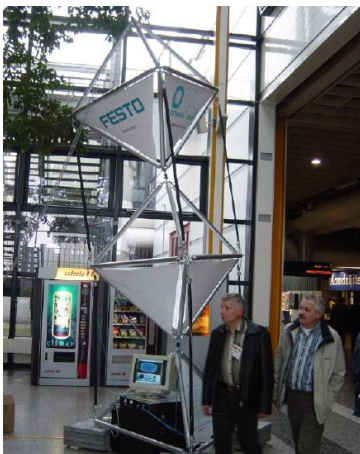
(Fig. 3.29) :Muscle Tower 1 the tower tilts according to the visitor's movement.
