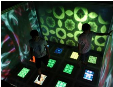
(Fig. 3.50) the installation where the floors are embedded with location sensors and the interactive walls are reconfigured according to the users choices
