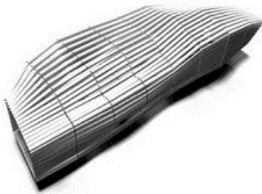
(Fig. 4.39) the exterior shape of e- motive house made of beams connected to each other with pneumatic muscles, which can be contracted and relaxed. Its form is a long movable space with two solid blocks on both ends
