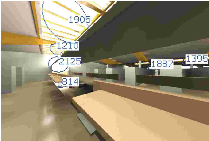
Figure 3-5 The lighting analysis allows qualification of luminance distribution by providing three dimensional displays that are made according to the eye's sensitivity.
