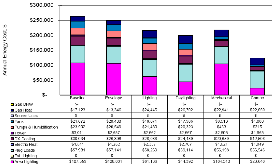
Figure 3-16 Annual Energy Cost Prediction for Various Energy Saving Design Strategies for the Old National Bancorp Headquarters (source: Old National Bancorp Headquarters URL: http://www.archenergy.com/services/sda/onb/ accessed July 2007)
