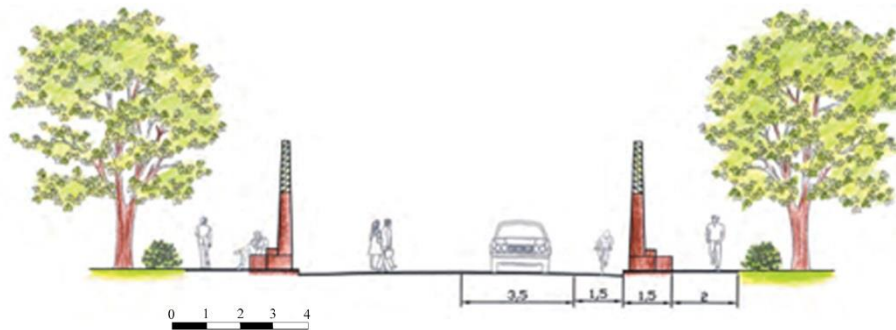
Fig. 9 Typical Campus Street Section at a Crosswalk in UNB Fredericton Campus. UNB Fredericton Campus Plan P.79
