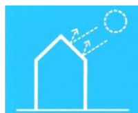
Figure (4.53): Actions promote the building's orientation in order enhance its exposure to daylighting Source: (IBA Hamburg, 2010)
