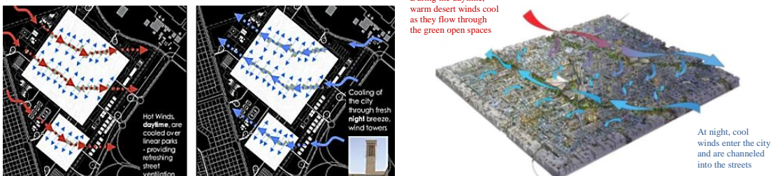
Figure (4.30): Approach adapts to nature wind in Masdar City Source: (Beglinger & Siegel, 2010)
