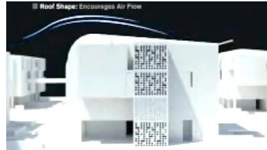
Figure (4.38): Example of the roof shape which encourages the air flow in Masdar City Source:(Archi Worlds, 2014)
