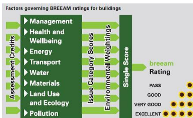
Figure (2.41): Factors governing BREEAM ratings for the building Source: (Building Research Establishment (BRE) Global, 2013)
