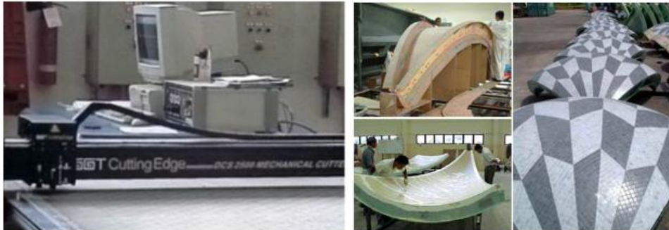
Fig. (3.110): Shots showing the Five-axis CNC milling machine and the manufacturing process of curved dome surfaces.
