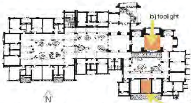
Floorplan of International Center for Desert Architecture and Appropriate Technologies. The highlighted entrance hall on the top has been equipped with a HOE-light guiding element, the room on the bottom has a light guiding window.
