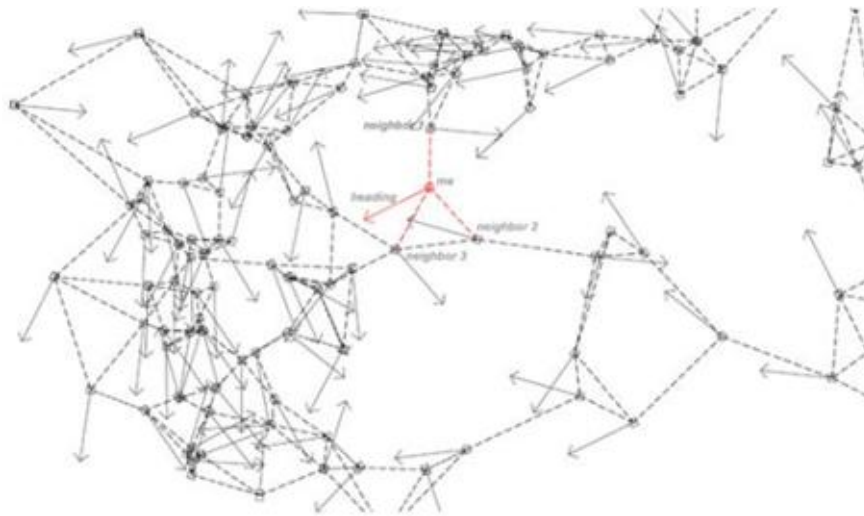
Figure 3.19 Diagram of Swarm Arrows represent each agent’s heading, dotted lines their closest neighbors. Source: - Carranza. P. M, Coates. P, “ The use of Swarm Intelligence to generate architectural form ”.
