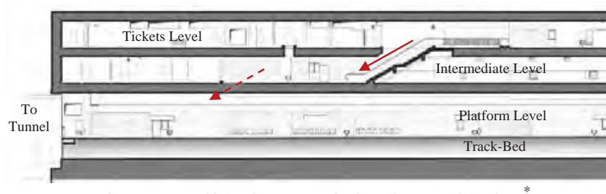
Figure 1-6: Half Section at a typical Underground Station.*
