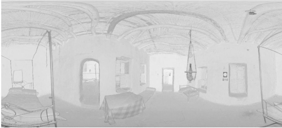
Figure 4.68 Laser scanning point clouds for the mayor's courthouse. Laser scanning measurements were used as an experimental measuring tool in Balat. One can get accurate measurements for vernacular buildings compared to manual sketches.
