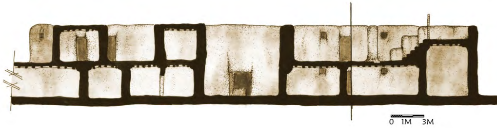
Figure 4.44 Section in the extended-family house showing internal heights.
