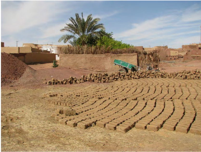
Figure 5.14 Mud brick drying in the sun. The bricks were flipped on all faces to ensure they dried completely from all directions.
