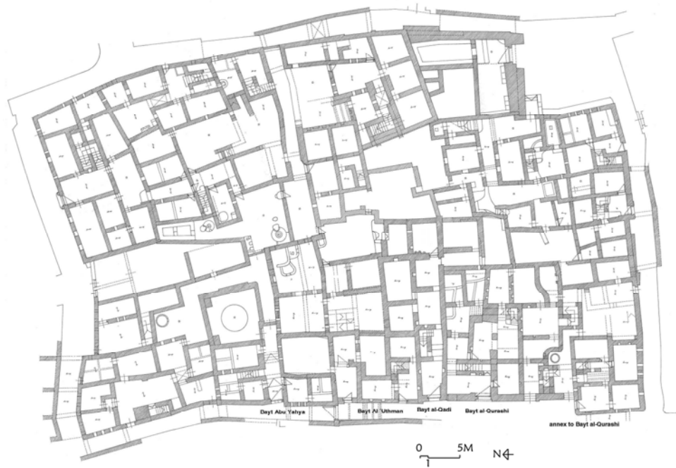
Figure 1.11 A ground floor plan of the Shihabiyya quarter in the old town of Al-Qasr. Source: Dakhla oasis project annual report 2008.
