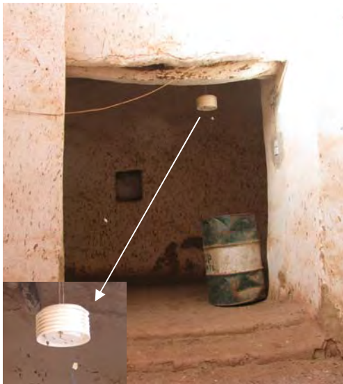
Figure 5.5 Outdoor temperature measuring loggers in Balat.
