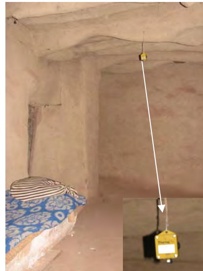
Figure 5.6 Indoor temperature measuring loggers in Balat.
