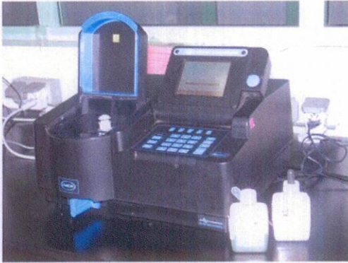
Plate 1. UV Spectro Photometer for sulphide, nitrogn and ammonia & phenol analyses.
