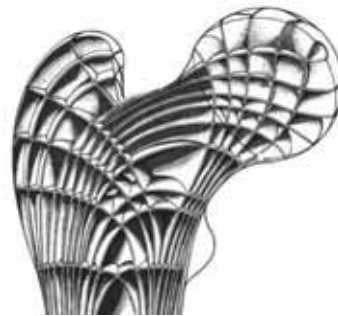
Fig. 1.32: Model showing direction of pure tension and pressure.
