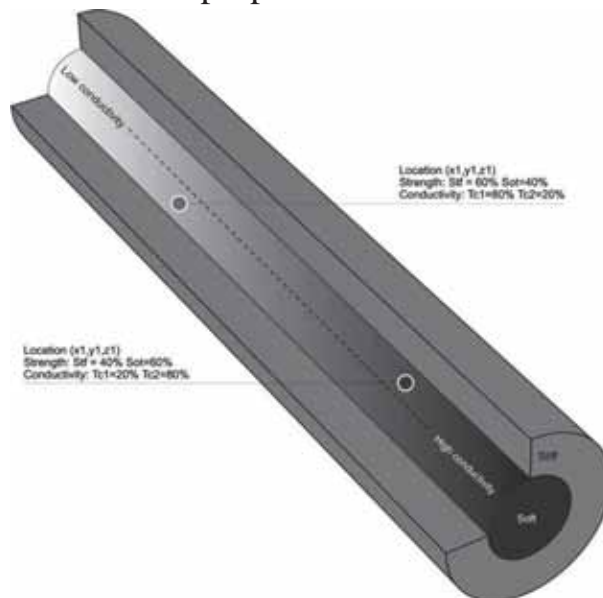
Fig. 2.28: Schematic 3D model illustrating multiple variable property representation.
