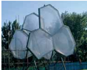
Fig. 2.35: Watercube physical prototype cells and ETFE cushions fabricated for the testing of environmental and structural behaviour.
