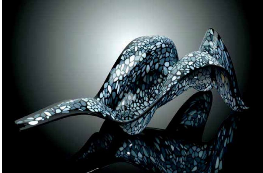
Fig. 2.13: Prototype for a Chaise Lounge, 2008, Boston Museum of Science. The chaise combines nature structural, environmental and performance by adapting its thickness, pattern density, stiffness and flexibility to load, curvature, and skin-pressured areas. It is patterned with 5 different materials color-coded by elastic moduli. Stiff (darker colored) and soft (lighter colored) materials are distributed according to the user's structural load distribution; Soft silicon is located in regions of higher pressure.
