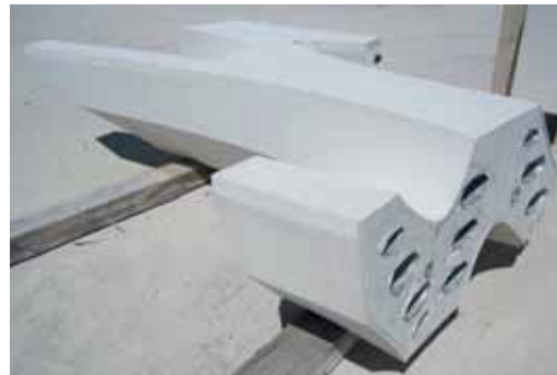
Fig. 4.34: Concrete Prototype Panel Showing Internal Steel & Cabling Routings penetrations.
