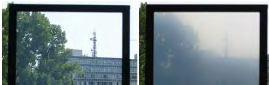
Figure (4-42) The Effect of Thermo Chromic Windows www.thermochromic-polymers.com/thermotropic/index.html
