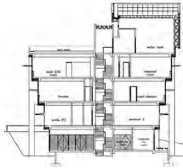
Figure (4-12) Self Shading by Segmented Profile in Pusat Tenaga Malaysia ( www.futurarc.com/previous_edition/zeroenergy.cfm )
