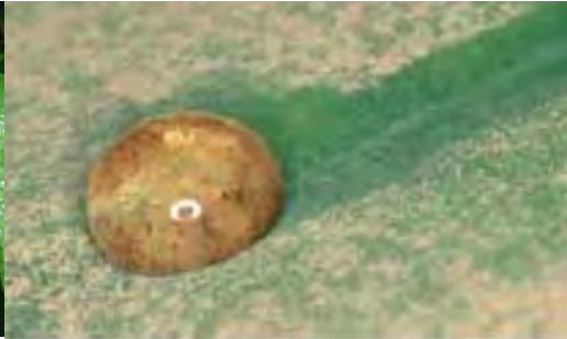
Figure (2-2) A Droplet Takes up the Dust Covering a Lotus Leaf. ( www.botanik.unibonn.de/system/lotus/en/prinzip_html.html )
