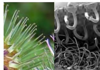
Figure (i-2): Closer Image to the Burr Seed (Left) and the Velcro Fastener Hooks and Loops (Right)
