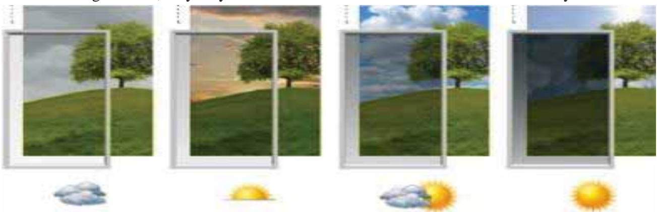
Figure 4- 41: The change of tinted color according to outdoor sun state Source: http://efficientdiy.com/portfolio/view-dynamic-glass-electronically-tinted-windows/
