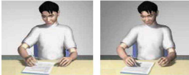
Figure 3- 14: Effect of light and shadow direction on a visual task Source: Good Lighting for Schools and Educational Establishments, p. 4
