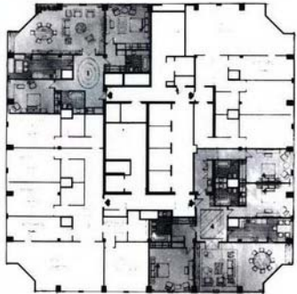
APARTMENT HOTEL: FLOORS 14-29 Typical Floor Plan 4 Apartments Total Area of Apartments per Floor 710sqm
