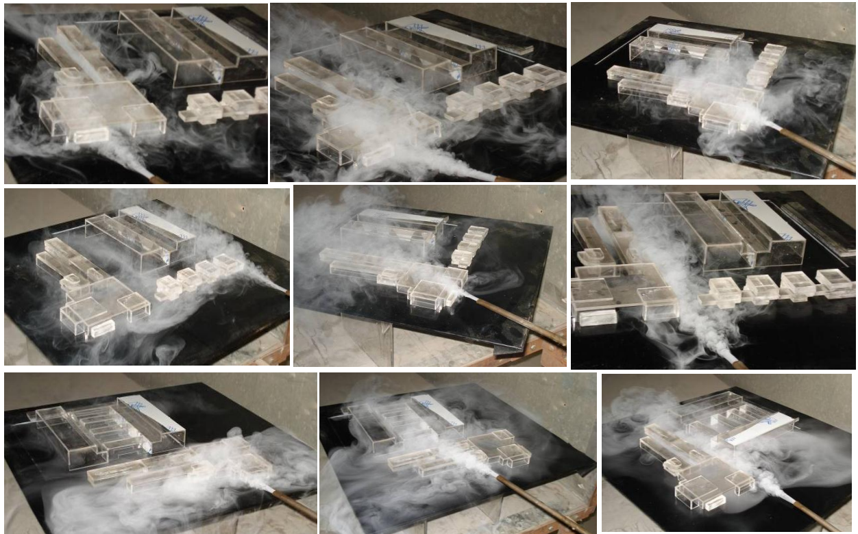
Fig. (2): Pictures of air flow through the model units, (Case No. 1).
