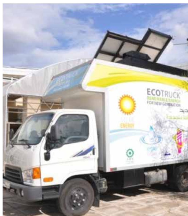
The Ecotruck is the first of its kind in Lebanon offering educational material and learning tools about renewable energy systems and applications. It is equipped with renewable energy technologies including solar water heating, micro wind, photovoltaic, and biomass systems
