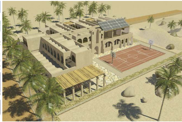
PV units as shade above the roof terraces, primary school in remote region (1 st prize competition, 2009)
